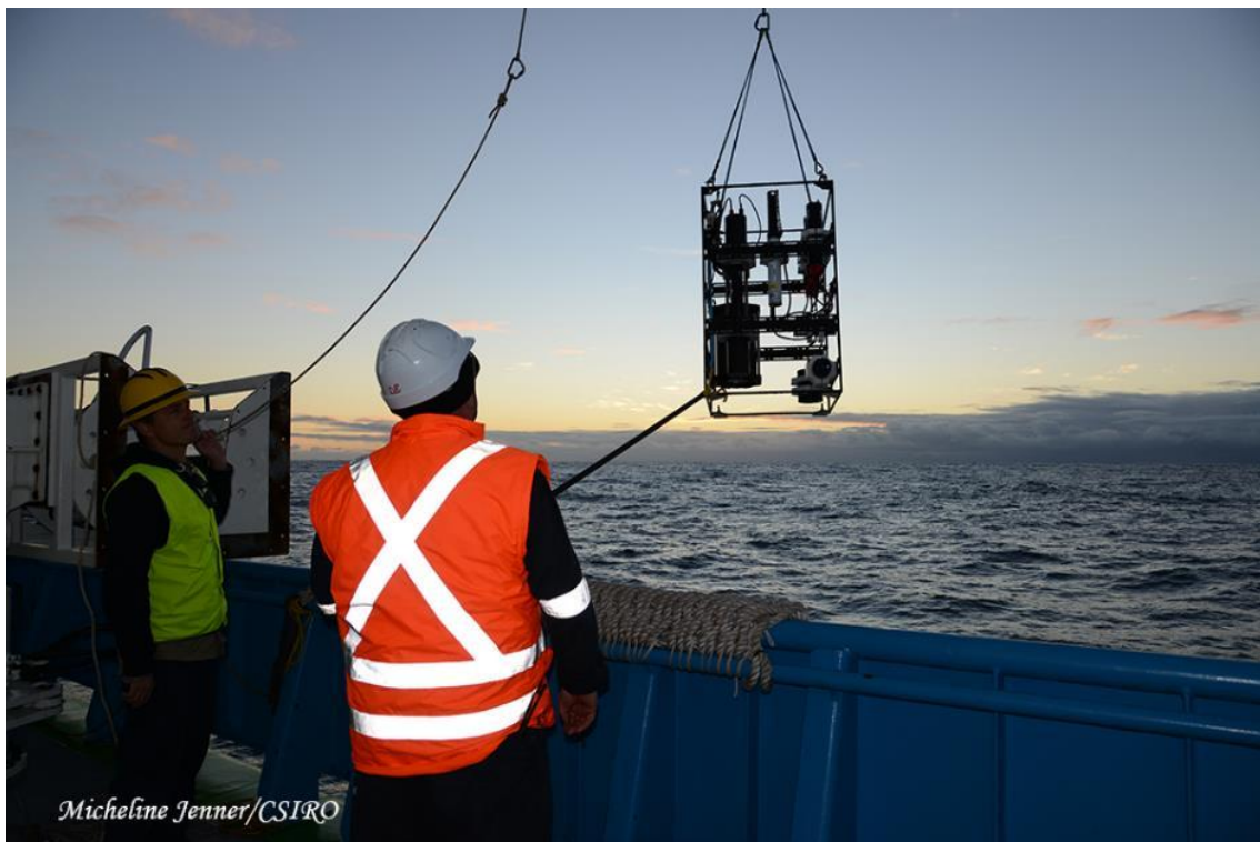
Photo 5: Retrieval of the Inherent Optical Properties package after a vertical deployment during Voyage IN2019_V03.
