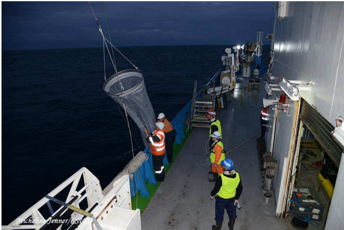
Photo 4. Retrieval of the Indian Ocean Standard net, a replica of the net used in the first International Indian Ocean Expedition during the 1960s, after a vertical haul on Voyage IN2019_V03.
