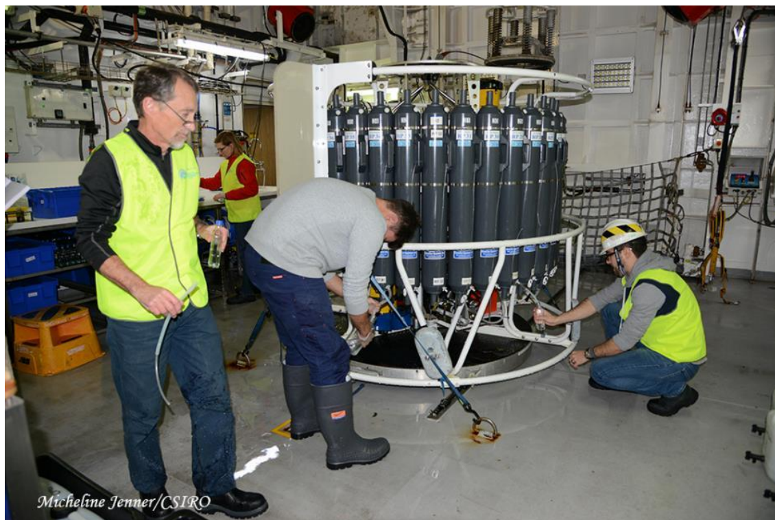
Photo 2. Casts of the CTD with its rosette of Niskin bottles to depths exceeding 5000m was a key activity at each of the stations along 110°E line during voyage IN2019_V03. Note the ADCP and UVP5 near the base of the rosette.
