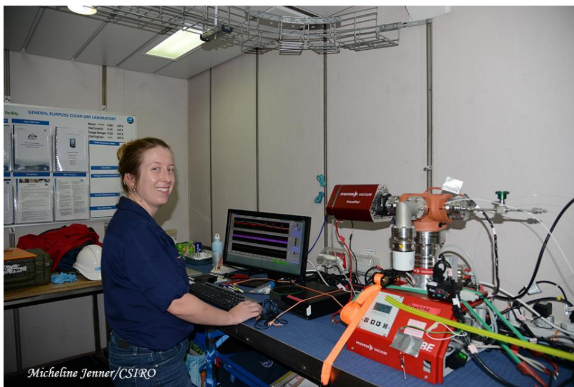
Photo 6. Dr Charlotte Robinson attending the Oxygen/Argon mass spectrometer for measuring net community production via the underway, throughflow seawater supply during Voyage IN2019_V03.
